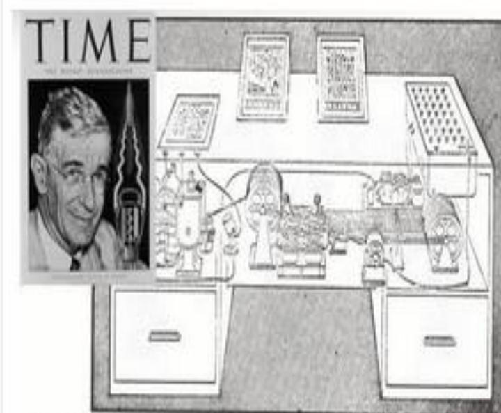
Memos in the form of a desk would instantly bring files and material on any subject to the operator's fingertips. Slanting translucent viewing screens magnify supermicrofilm filed by code numbers. At left is a mechanism which automatically photographs longhand notes, pictures and letters, then files them in the desk for future reference (TIME 1943), p. 123.
